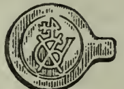
SINGLE-DISC CLIP AFTER CLOSING, SHOWING DEVICE STAMPED ON END OF TONGUE.
